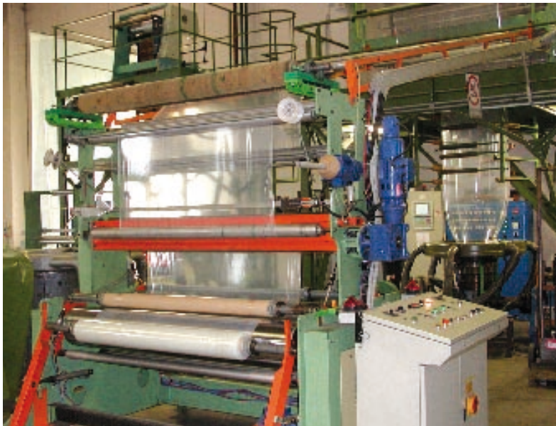
Blow extrusion pilot plant at P.A.T.I S.p.A.
