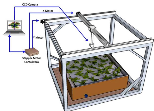
Fig. 1. Schematics of the machine vision-guided plant monitoring system.
