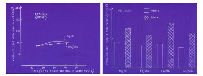
Growth data for Petunias comparing double IR film to double non-IR with regard to leaf index for one variety and dry weights for two varieties grown in each of the four test greenhouses
