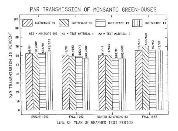
Fig. 3. PAR Transmission of all Test Houses in all Test Periods
