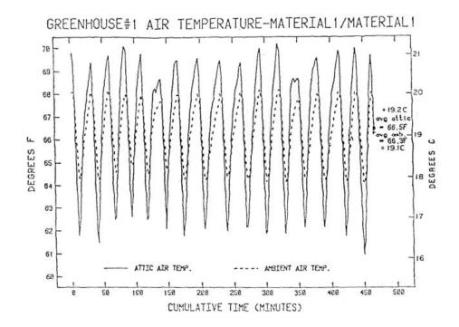
Fig. 5. Detailed Temperature Data Showing Heater Cycling Greenhouse 1
