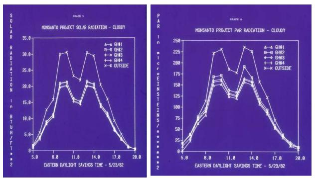
Representative total solar radiation and PAR radiation outside and inside each greenhouse for a partially cloudy day
