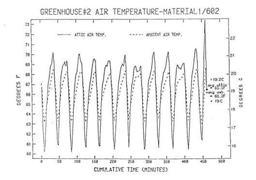
Fig. 6. Detailed Temperature Data Showing Heater Cycling Greenhouse 2
