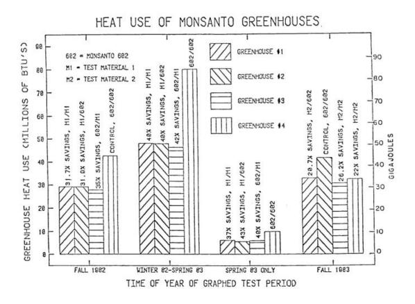
Fig. 4. Total Energy Consumption for Four Test Periods
