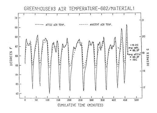
Fig. 7. Detailed Temperature Data Showing Heater Cycling Greenhouse 3
