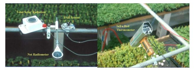
Radiation sensor array inside the greenhouse that measure: Total solar spectrum, PAR and net thermal radiation from crop canopy <u>Return to sensor description</u> Infrared thermometer Return to text IR thermometer
