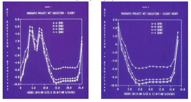
Representative net radiation for the test houses day and night on the left and expanded night scale on the right
