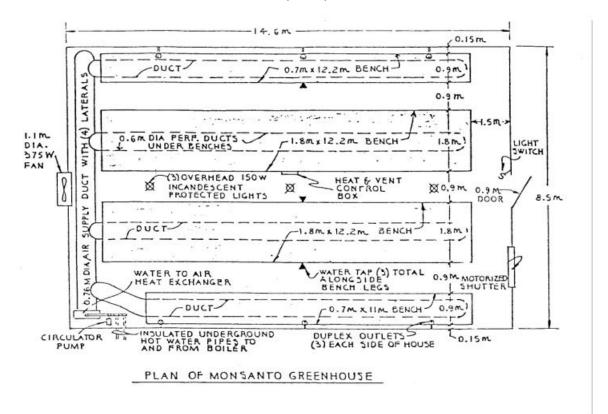
Fig. 2. Test Greenhouse Layout
