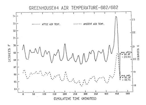
Fig. 8. Detailed Temperature Data Showing Heater Cycling Greenhouse 4
