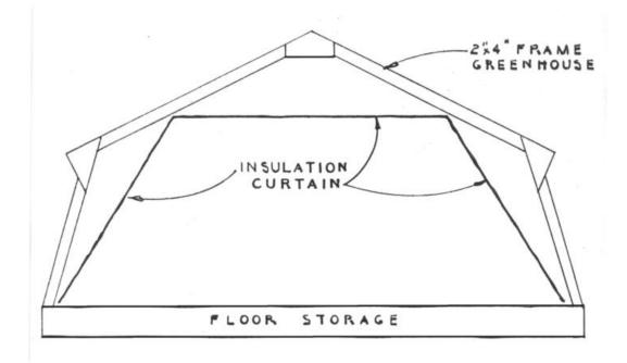
Fig. 2 Planar Insulation System for Small Prototype Greenhouse
