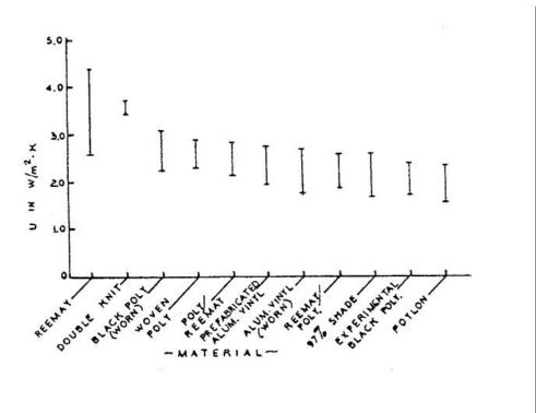
Fig. 4 Heat Transfer Coefficients for Selected Curtain Types
