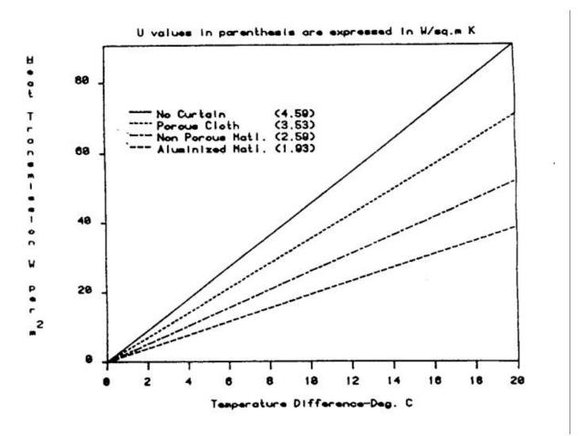
Fig. 5 Heat Transmission of Various Curtain Types
