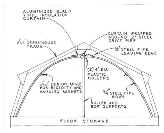
Fig. 1 Curved Curtain Insulation System for Small Prototype Greenhouse
