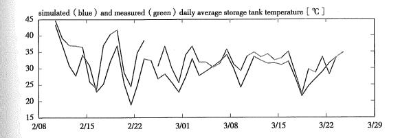
shown in the following graph were obtained. The simulation was run with all parameters equal to the parameters found during the tuning on the measured data. The weather data for Shouguang were not available for this period so therefore the weather data from Qingdao International airport were used.
