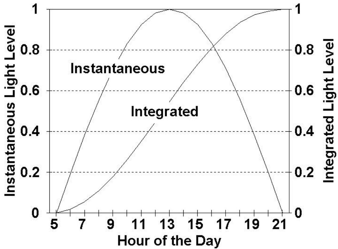
Figure 1. Normalized instantaneous and integrated light levels (sunlight only) for a clear and sunny day with a 16-hour light period.
