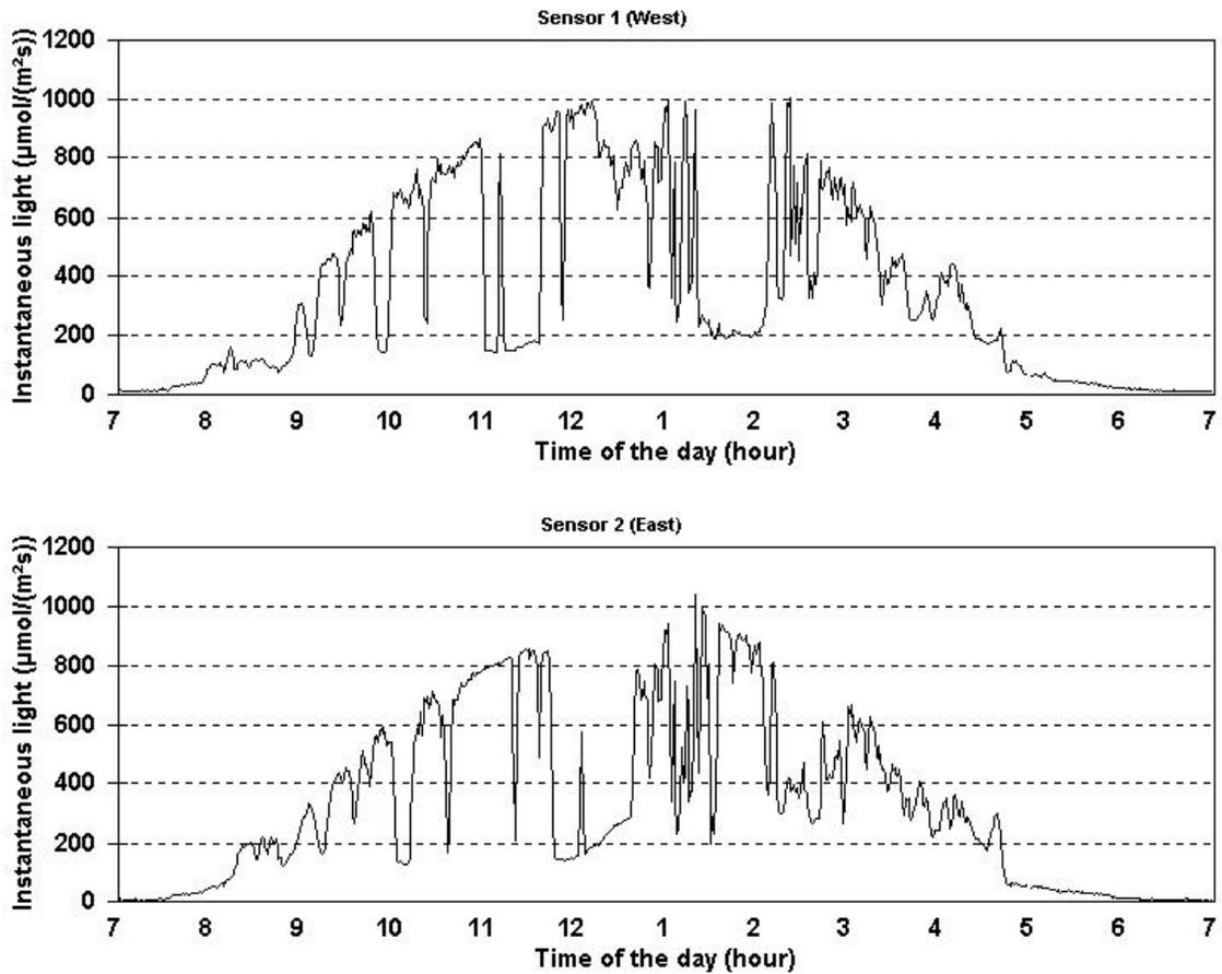
Figure 3. Instantaneous light levels measured with two light sensors in two different locations inside a greenhouse and for a 12-hour measuring period. Note that the sensors are, for the most part, not shaded (by the greenhouse structure) at the same time so that their averaged reading gives a better approximation of the overall light environment in the greenhouse.
